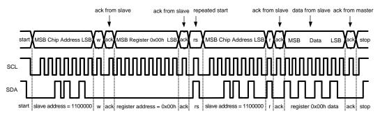
Figure 32. Example I<sup>2</sup>C Read Cycle
