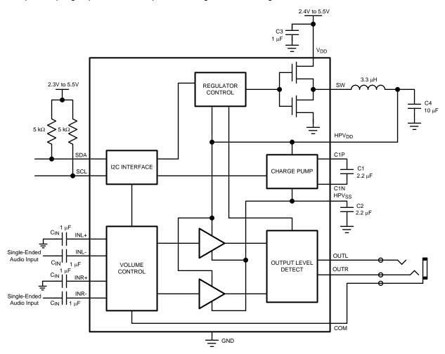
Figure 36. Single-Ended Input Configuration
