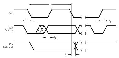
Figure 29. I<sup>2</sup>C Timing Diagram
