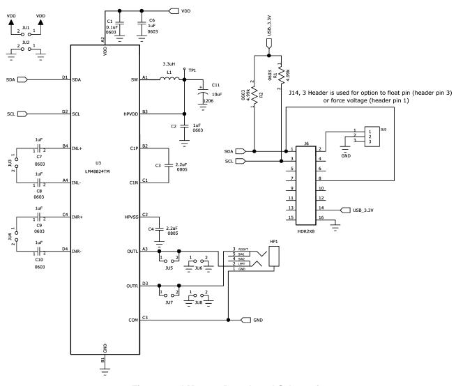
Figure 37. LM48824 Demoboard Schematic
