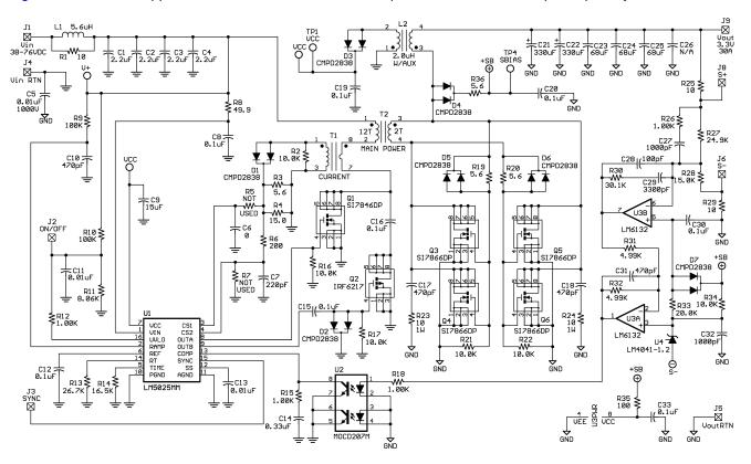
Figure 21. Application Circuit
