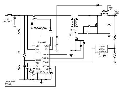
Figure 13. Simplified Active Clamp Forward Power Converter
