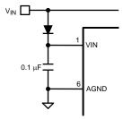
Figure 26. Input Blocking Diode for VCCX > VIN
