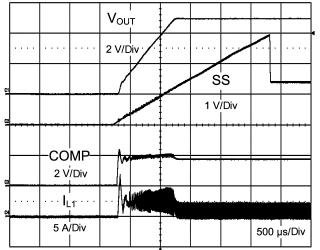
Figure 41. Short Circuit Recovery Into Resistive Load With C7 = 1 µF and D2 Installed
