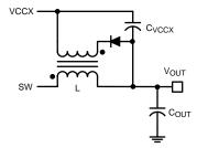
Figure 25. VCCX Bias Supply with Additional Inductor Winding
