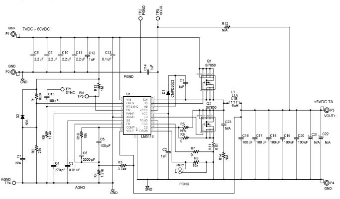
Figure 33. 5-V 7-A Typical Application Schematic
