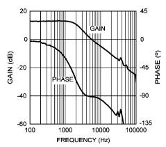
Figure 35. Modulator Gain and Phase
