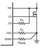
Figure 30. R<sub>DS(ON)</sub> Current Sensing without Diode Emulation
