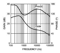
Figure 36. Error Amplifier Gain and Phase
