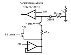
Figure 32. Diode Emulation Control
