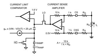
Figure 31. Current Limit and Ramp Circuit
