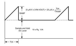
Figure 29. Composition of Current Sense Signal
