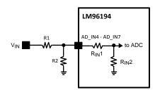
Figure 7. Internal Resistors,  $R_{IN}1 + R_{IN}2$
