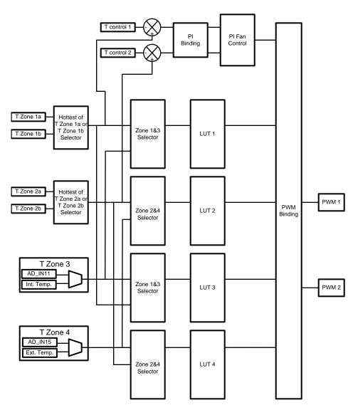
Figure 11. LUT and PI controller high level block diagram
