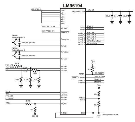
Figure 3. Recommended implementation without thermal diode connections
