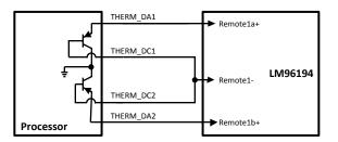
**Note:** 100 pF cap across each thermal diode is optional and should be placed close to the LM96194, if used. The maximum capacitance between thermal diode pins is 300 pF.
