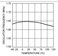
Figure 7. Oscillator Frequency vs Temperature - "X"
