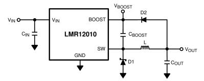
Figure 15. V<sub>OUT</sub> Charges C<sub>BOOST</sub>
