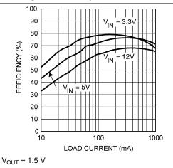
Figure 5. Efficiency vs Load Current - "X"
