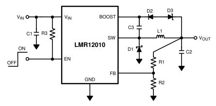
Figure 19. V<sub>BOOST</sub> Derived From Series Zener Diode (V<sub>OUT</sub>)
