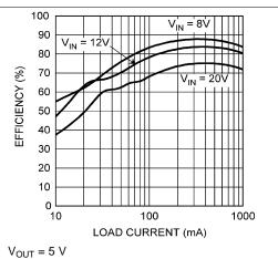
Figure 2. Efficiency vs Load Current - "Y"
