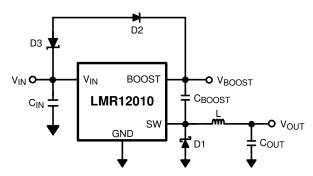
Figure 16. Zener Reduces Boost Voltage From VIN
