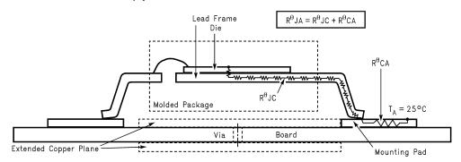
Figure 25. Cross-Sectional View of Integrated Circuit Mounted on a Printed Circuit Board.
