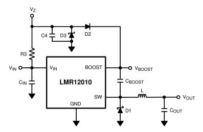
Figure 17. Boost Voltage Supplied From the Shunt Zener on  $\rm V_{IN}$
