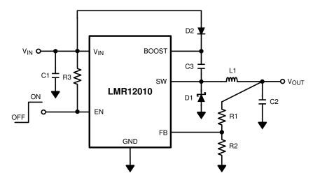
Figure 18.  $V_{BOOST}$  Derived From  $V_{IN}$
