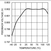
Figure 11. V<sub>FB</sub> vs Temperature
