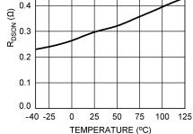
Figure 12. R<sub>DSON</sub> vs Temperature
