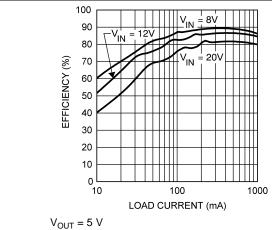
Figure 1. Efficiency vs Load Current - "X"
