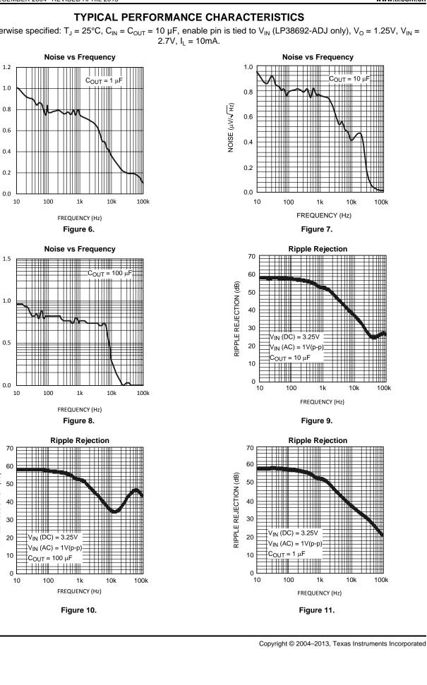
Unless otherwise specified:  $T_J = 25^{\circ}C$ ,  $C_{IN} = C_{OUT} = 10 \ \mu$ F, enable pin is tied to  $V_{IN}$  (LP38692-ADJ only),  $V_O = 1.25V$ ,  $V_{IN} = 1.25$
