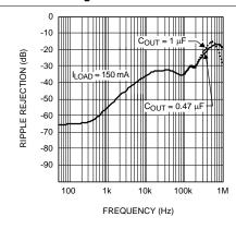
Figure 9. Power Supply Rejection Ratio
