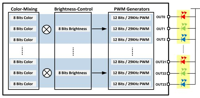
图 9. PWM Control Scheme for Each Channel
