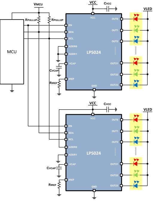
图 61. Driving Dual LP5024 Application Example
