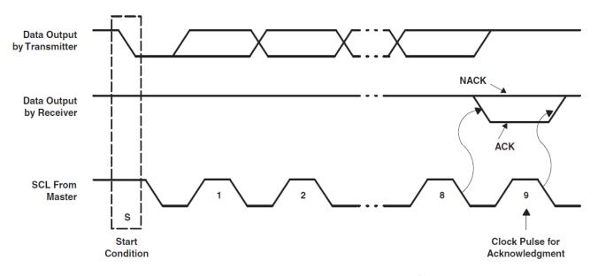
图 18. Acknowledge and Not Acknowledge on I<sup>2</sup>C Bus
