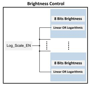
图 10. Logarithmic- or Linear-Scale Intensity Control
