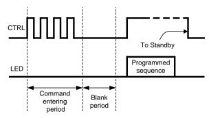
Figure 12. Delayed Run-Once Command
