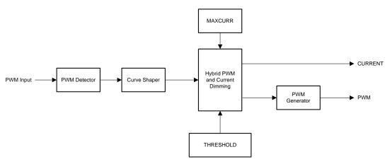
Figure 24. BRTMODE = 00 Brightness Control
