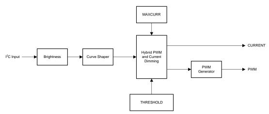
Figure 25. BRTMODE = 01 Brightness Control
