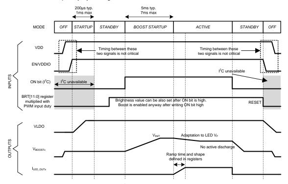
Figure 36. Start-up and Shutdown with I<sup>2</sup>C + PWM Input Brightness Control (BRTMODE = 01b)
