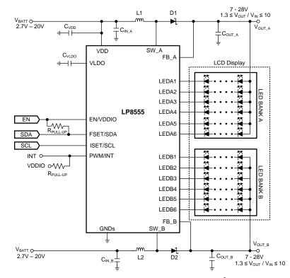
Figure 51. Application Example With 12 LED Strings, I<sup>2</sup>C Brightness Control
