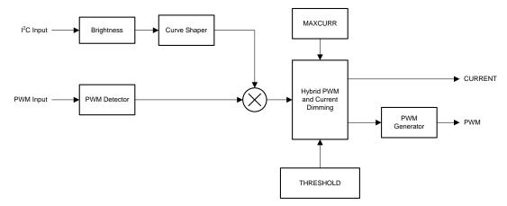
Figure 27. BRTMODE = 11 Brightness Control
