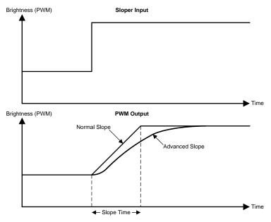
Figure 32. Sloping Principle
