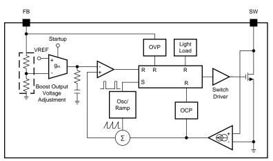
Figure 20. Boost Converter Functional Block Diagram
