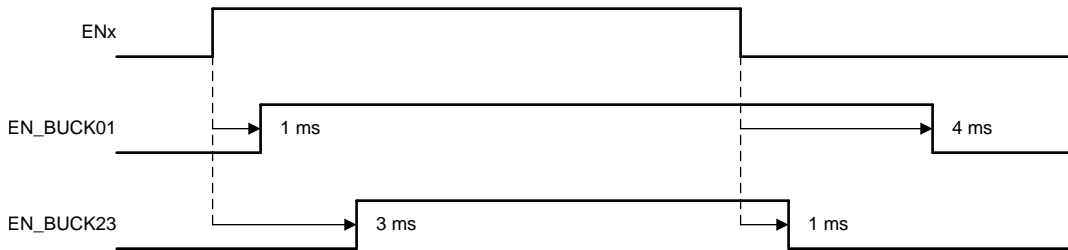
图 16. Typical Start-Up and Shutdown Sequencing
