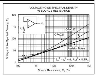
Figure 42. Noise Performance of the OPA2211 and OPA227 in Unity-Gain Buffer Configuration
