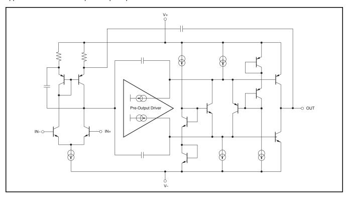
Figure 40. OPA2211 Simplified Schematic
