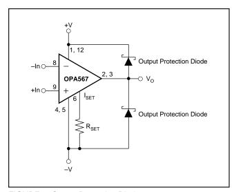
FIGURE 5. Output Protection Diode.
