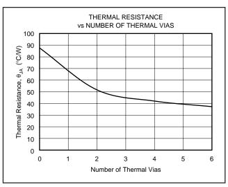
FIGURE 11. Thermal Resistance vs Number of Thermal Vias.
