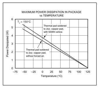
FIGURE 10. Maximum Power Dissipation vs Temperature.
