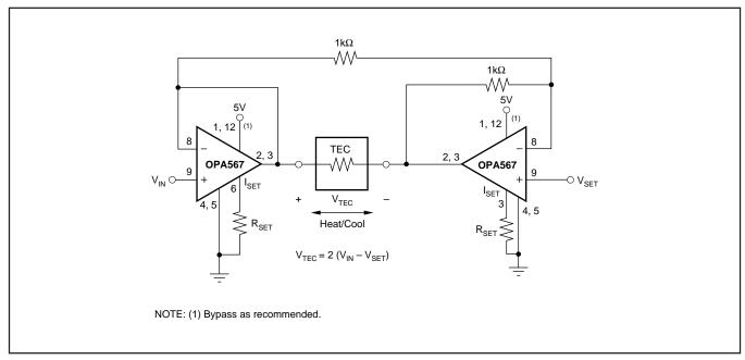
FIGURE 14. Bridge-Tied Load Driver.
