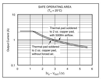
FIGURE 7. Safe Operating Area at Room Temperature.
