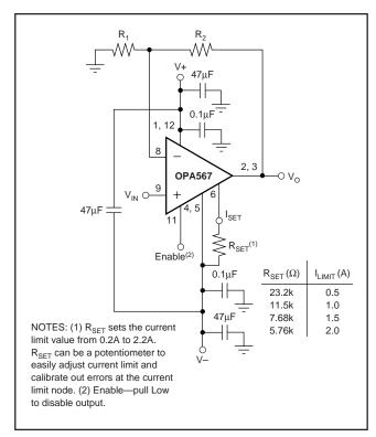
FIGURE 1. Basic Connections.
