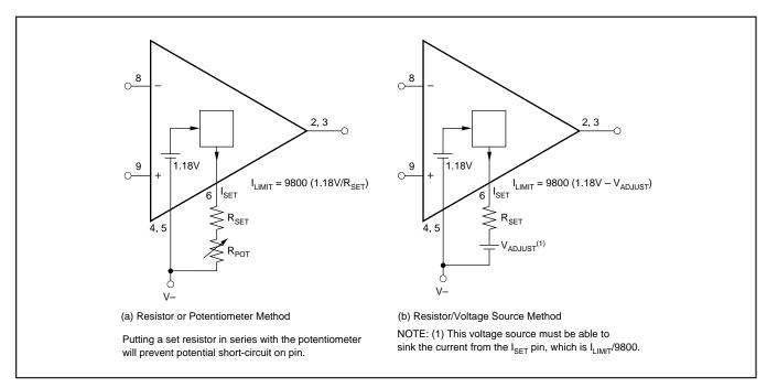
FIGURE 2. Setting the Current Limit—Resistor Method.
