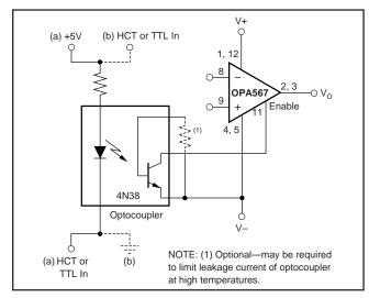
FIGURE 4. OPA567 Shutdown Configuration for Dual Supplies.
