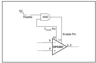
FIGURE 6. Enable/Shutdown Control Using T<sub>FLAG</sub> Pin and External Control Signal.
