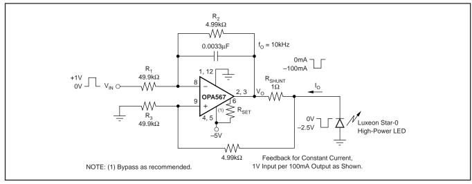
FIGURE 13. Grounded Anode LED Driver.
