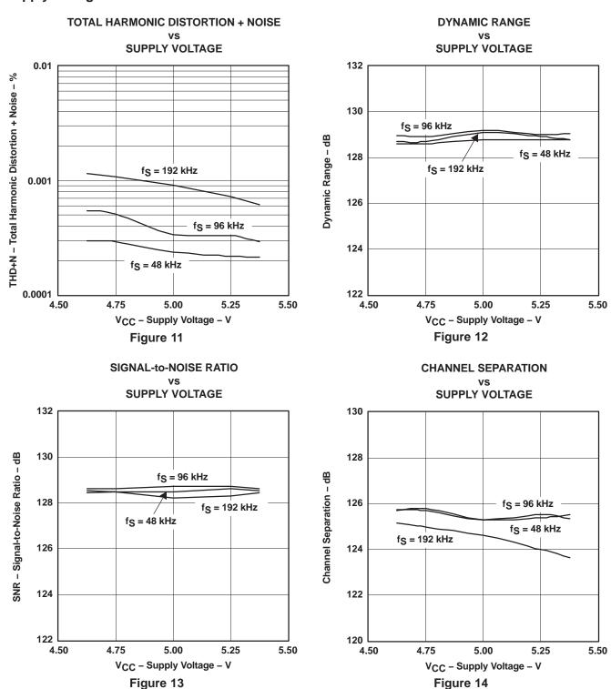
NOTE: PCM mode,  $T_A = 25$ °C,  $V_{DD} = 3.3$  V, measurement circuit is Figure 37 ( $V_{OUT} = 4.5$  V rms).
