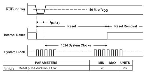
Figure 26. External Reset Timing
