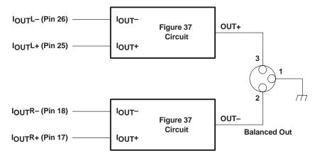
Figure 39. Measurement Circuit for Monaural Mode
