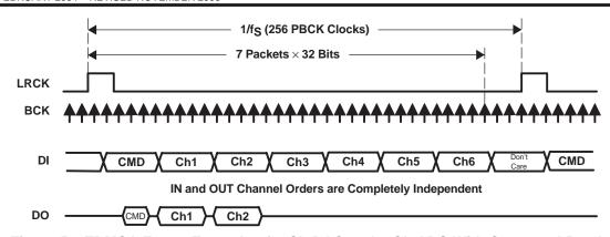
Figure 59. TDMCA Frame Example of 6-Ch DAC and 2-Ch ADC With Command Read
