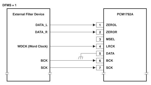
Figure 40. Connection Diagram for External Digital Filter (Internal DF Bypass Mode) Application
