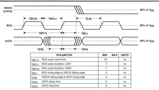
Figure 42. Audio Interface Timing for External Digital Filter (Internal DF Bypass Mode) Application
