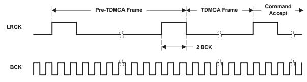
Figure 54. LRCK and BCK Timing of Determination TDMCA Mode
