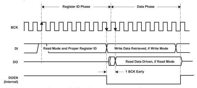
Figure 60. TDMCA Write and Read Operation Timing
