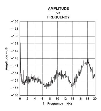
Figure 23. -150-dB Output Spectrum, DSD Mono Mode
