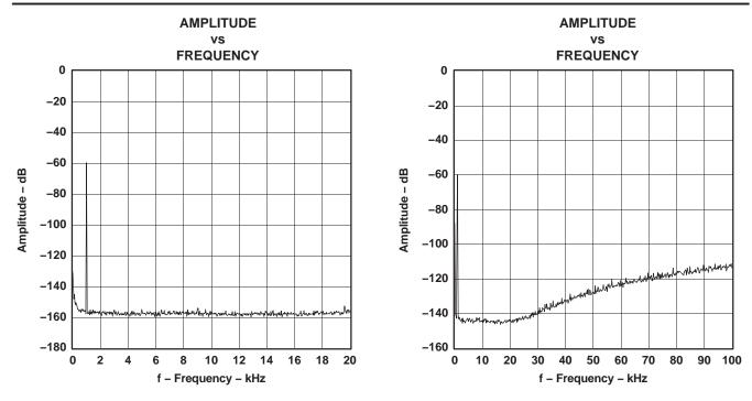
Figure 19. –60-dB Output Spectrum, BW = 20 kHz Figure 20. –60-dB Output Spectrum, BW = 100 kHz NOTE: PCM mode,  $f_S = 48$  kHz, 32,768 point 8 average,  $T_A = 25^{\circ}$ C,  $V_{DD} = 3.5$  V  $V_{CC} = 5$  V, measurement circuit is Figure 37.
