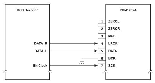
Figure 43. Connection Diagram in DSD Mode
