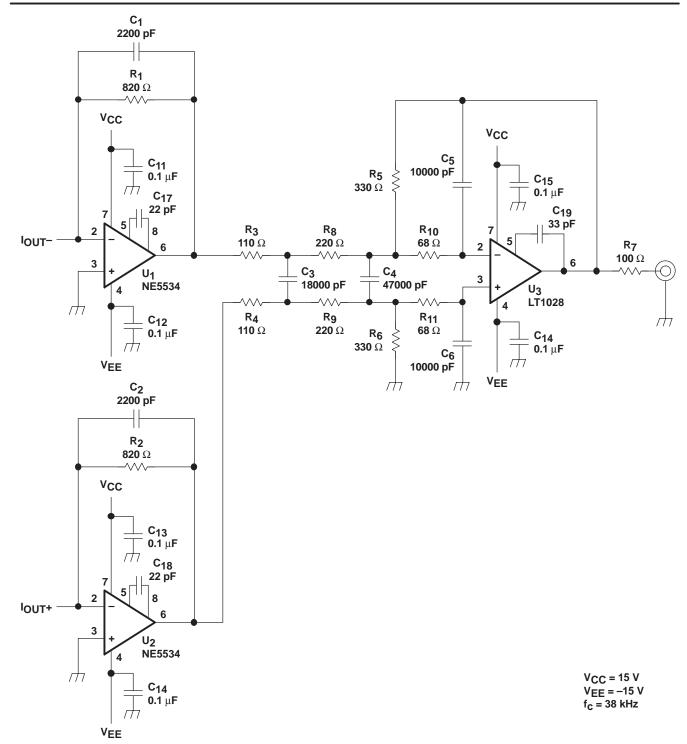
Figure 38. Measurement Circuit for DSD
