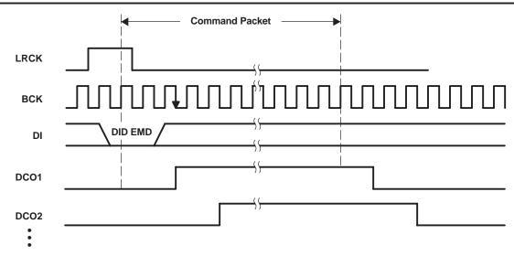
Figure 63. DCO Output Timing With Skip Operation (for Command Packet 1)
