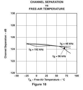
NOTE: PCM mode,  $V_{DD}$  = 3.3 V,  $V_{CC}$  = 5 V, measurement circuit is Figure 37 ( $V_{OUT}$  = 4.5 V rms).
