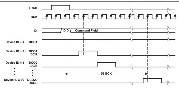
Figure 57. Device ID Determination Sequence
