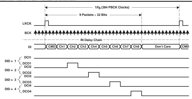
Figure 61. DCO Output Timing of TDMCA Mode Operation
