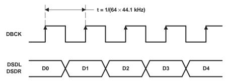
Figure 44. Normal Data Output Form From DSD Decoder
