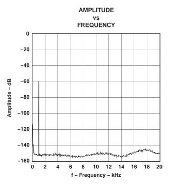
Figure 22. -60-dB Output Spectrum, DSD Mode
