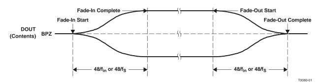
Figure 18. Fade-In and Fade-Out Operations
