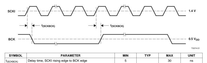
NOTE: Timing measurement reference level is 1.4 V for input and 0.5 V<sub>DD</sub> for output. Load capacitance of BCK is 20 pF. This timing is applied when SCKI frequency is less than 25 MHz.
