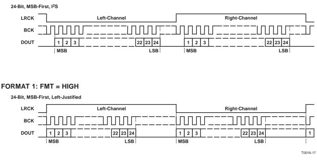
Figure 21. Audio Data Format (LRCK and BCK Work as Inputs in Slave Mode and as Outputs in Master Mode)
