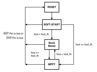
Figure 4. High Level State Diagram for Startup
