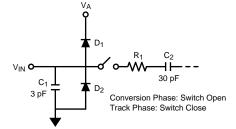
Figure 7. Equivalent Input Circuit
