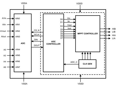
Figure 1. Block Diagram
