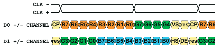
图 8-5. Data and Clock Input in 2-ChM (LS0 = high; LS1 = low)
