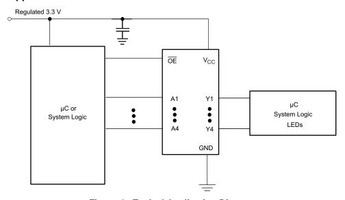
Figure 4. Typical Application Diagram
