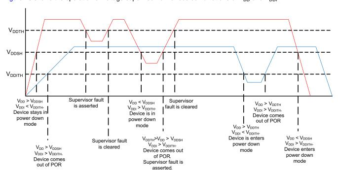
Figure 18. Voltage Supervisor Operation
