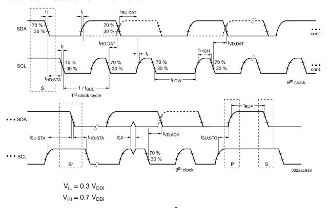
Figure 2. Parameter Measurement Information for I<sup>2</sup>C Timing Characteristics and Requirements
