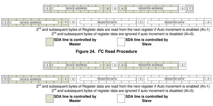
Figure 25. I<sup>2</sup>C Read Procedure with Repeated Start
