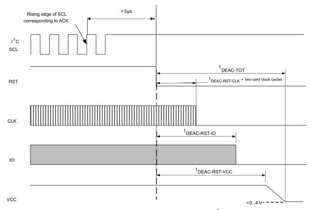
Figure 8. Card Deactivation Sequence Initiated by I<sup>2</sup>C Command
