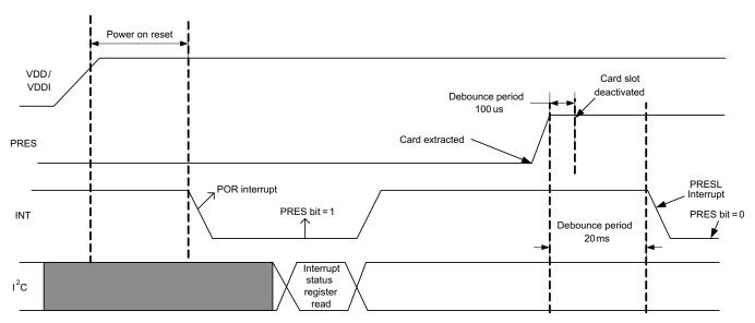
Figure 14. Device Power up with Card Inserted In System - High to Low PRES Topology
