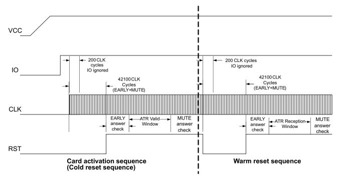
Figure 6. Asynchronous Activation and Warm Reset Sequence
