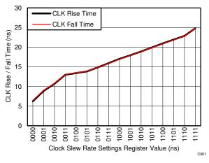
$C_{\text{L}} = 30~\text{pF}$  Figure 1. CLK Rise/Fall Time vs Clock Slew Rate Settings Register Value
