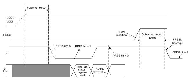
Figure 11. Device power up without card inserted in system - Low to High PRES Topology
