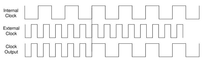
Figure 16. Output CLK Frequency Transition When Switching From External Clock to Internal Clock
