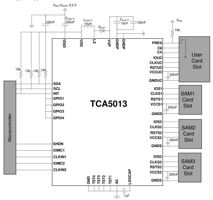
Figure 26. POS Terminal Typical Application
