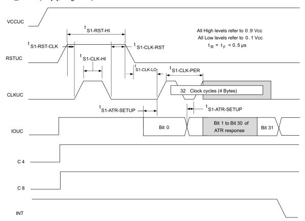
Figure 4. Synchronous Type 1 Activation Sequence
