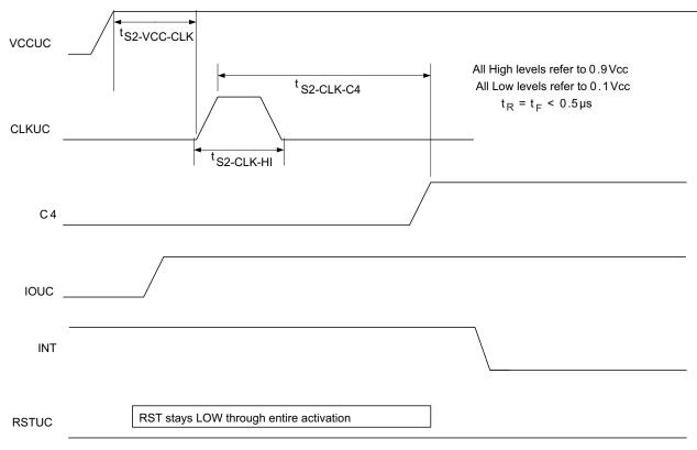
Figure 5. Synchronous Type 2 Activation Sequence
