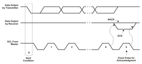
Figure 22. Acknowledgment on I<sup>2</sup>C Bus
