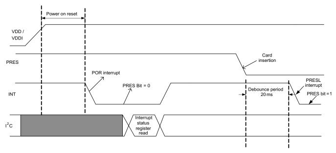
Figure 12. Device power up without card inserted in system - High to Low PRES Topology
