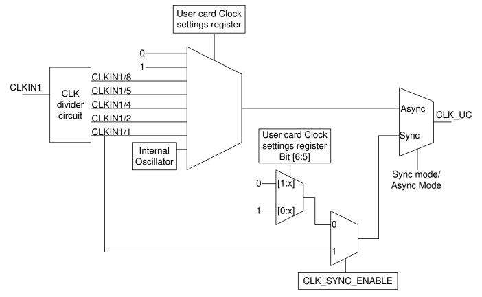
Figure 17. Clock Muxing Logic in Synchronous Mode
