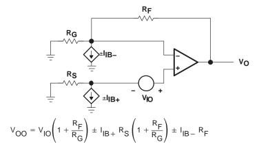
Figure 47. Output Offset Voltage Model
