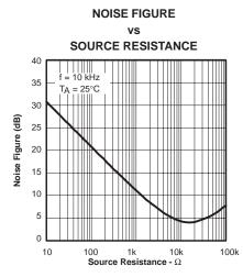
Figure 44. Noise Figure vs Source Resistance
