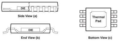
NOTE A: The thermal pad is electrically isolated from all terminals in the package.
