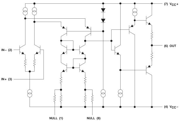
Figure 42. THS405x Simplified Schematic
