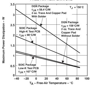
NOTE A: Results are with no air flow and PCB size =  $3"\times 3"$
