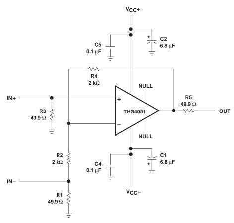
Figure 58. THS4051 Evaluation Board Schematic
