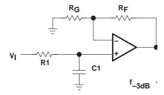
Figure 49. Single-Pole Low-Pass Filter
