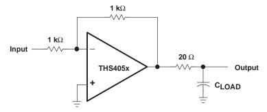
Figure 45. Driving a Capacitive Load
