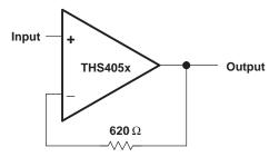
Figure 48. Noninverting, Unity Gain Schematic
