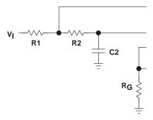
Figure 50. 2-Pole Low-Pass Sallen-Key Filter
