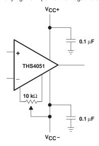
Figure 46. Offset Nulling Schematic
