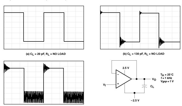
Figure 41. Effect of Capacitive Loads and Test Circuit
