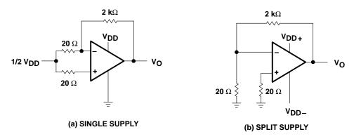
Figure 2. Noise-Test Circuit
