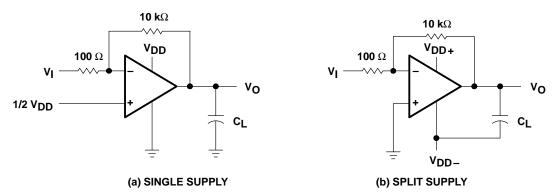
Figure 3. Gain-of-100 Inverting Amplifier
