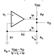
$I_p$  = Pullup current required by the operational amplifier (typically 500  $\mu$ A)
