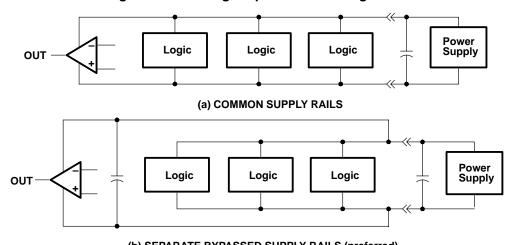
(b) SEPARATE BYPASSED SUPPLY RAILS (preferred)
