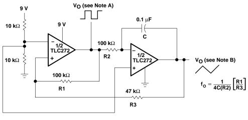
NOTES: A.  $V_{O(PP)} = 8 \text{ V}$ B.  $V_{O(PP)} = 4 \text{ V}$
