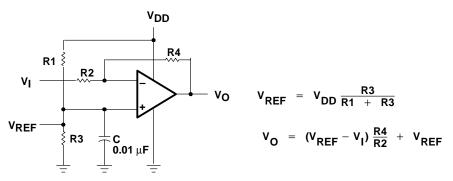
Figure 38. Inverting Amplifier With Voltage Reference
