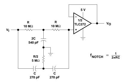
Figure 49. Single-Supply Twin-T Notch Filter
