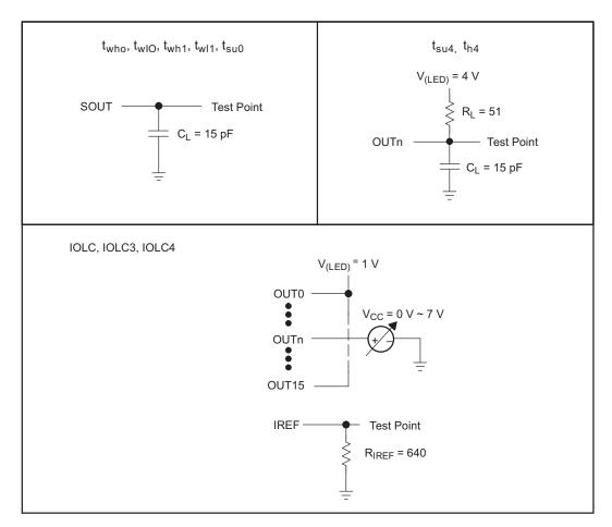
Figure 2. Parameter Measurement Circuits
