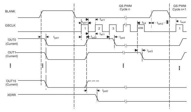
Figure 15. Grayscale PWM Cycle Timing Chart
