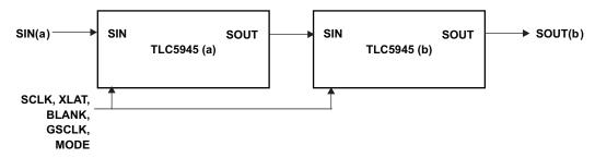
Figure 7. Cascading Two TLC5945 Devices
