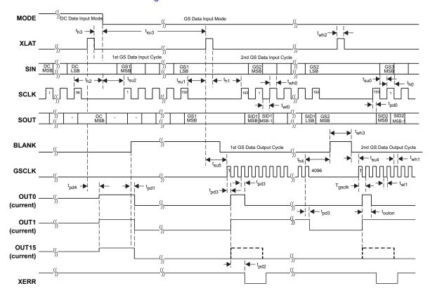
Figure 6. Serial Data Input Timing Chart
