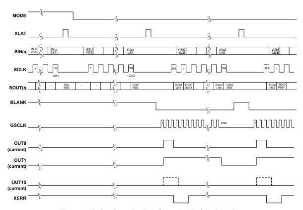
Figure 8. Timing Chart for Two Cascaded TLC5945 Devices
