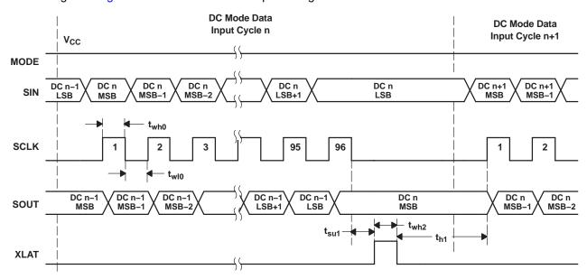
Figure 10. Dot Correction Data Input Timing Chart
