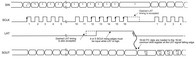
Figure 24. FC Data Read (READFC) Command Timing Diagram
