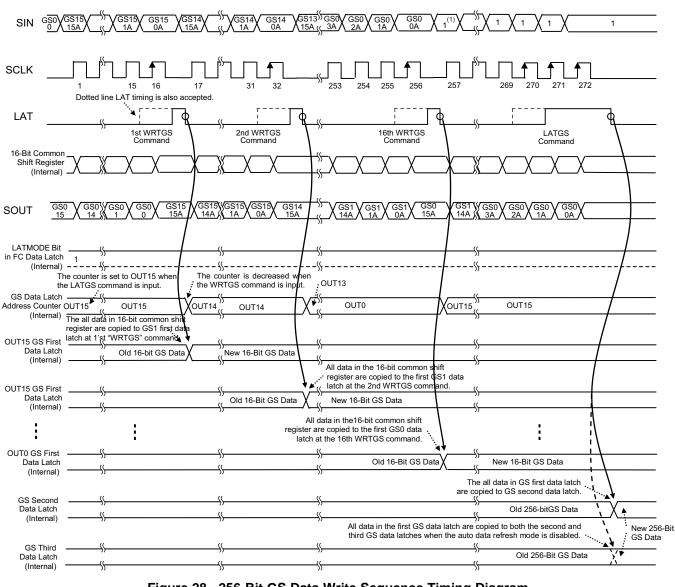
Figure 28. 256-Bit GS Data Write Sequence Timing Diagram (16 × WRTGS + 1 LATGS, LATMODE = 1)
