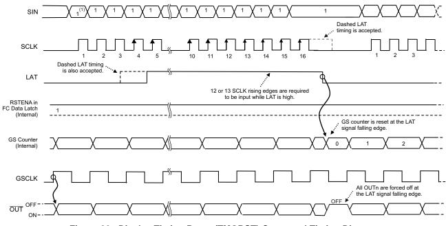
Figure 26. Display Timing Reset (TMGRST) Command Timing Diagram
