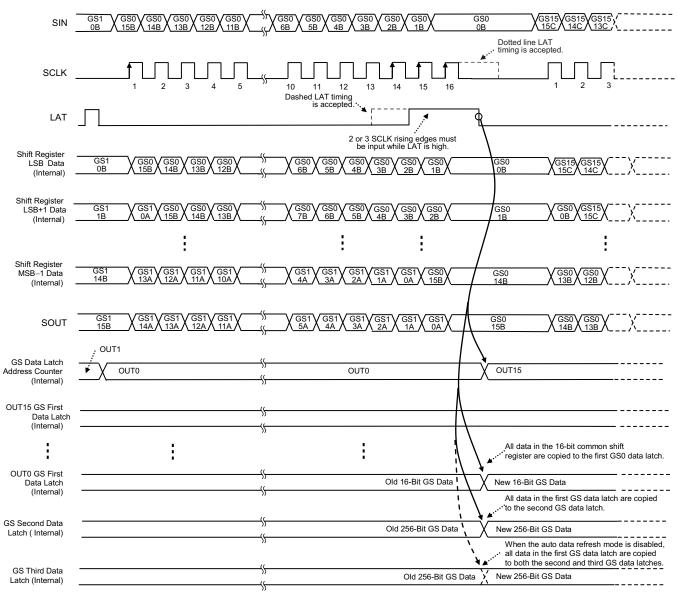
Figure 23. 256-Bit GS Data Latch (LATGS) Command (LATMODE = 0)
