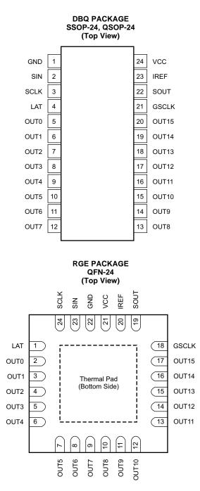
NOTE: The thermal pad is not internally connected to GND. The thermal pad must be connected to GND via the printed board circuit (PCB) pattern.
