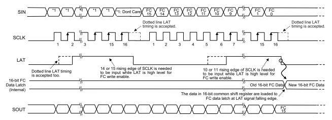
Figure 25. FC Data Write Enable (FCWRTEN) and FC Data Write (WRTFC) Command Timing Diagram
