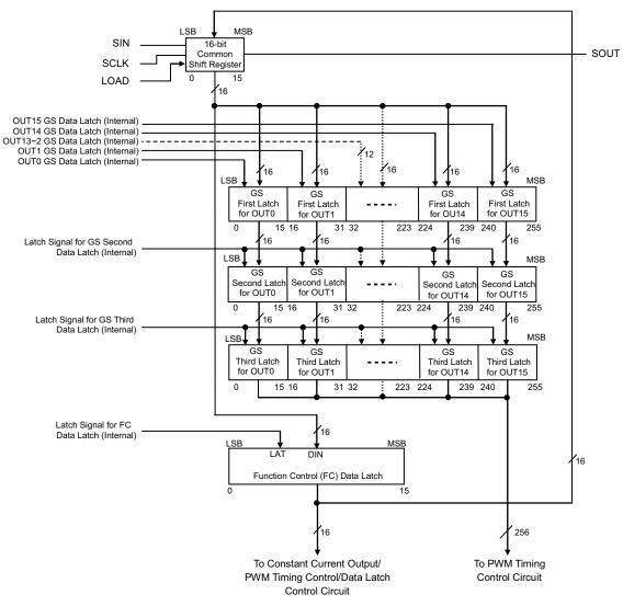
Figure 21. Shift Register and Data Latch Configuration
