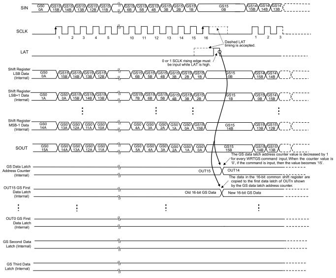
Figure 22. 16-Bit GS Data Write (WRTGS) Command
