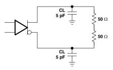
Figure 8. Transmitter Test Setup
