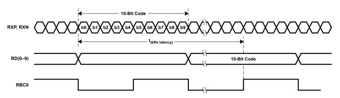
Figure 7. Receiver Latency, TBI Normal Mode Shown
