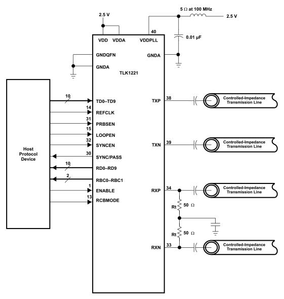
Figure 12. Typical Application Circuit (AC Mode)
