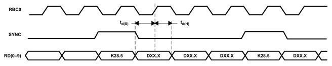
Figure 3. Synchronous Timing Characteristic Waveforms (TBI Full-Rate Mode)
