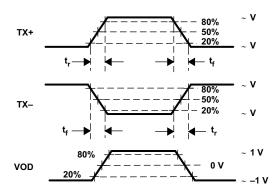
Figure 6. Differential and Common-Mode Output Voltage Definitions
