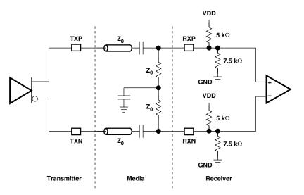
Figure 11. High-Speed I/O AC-Coupled Mode
