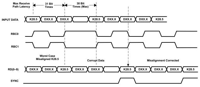
Figure 4. Word Realignment Timing Characteristic Waveforms
