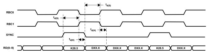
Figure 2. Synchronous Timing Characteristic Waveforms (TBI Half-Rate Mode)
