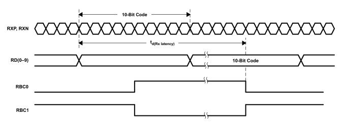
Figure 5. Receiver Latency, TBI Half-Rate Mode Shown
