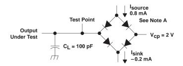
NOTE A: Equivalent load circuit of the Teradyne A580 tester for timing parameter measurement.
