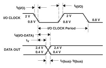
Figure 7. I/O CLOCK and DATA OUT Voltage Waveforms
