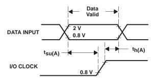
Figure 5. DATA INPUT and I/O CLOCK **Voltage Waveforms**
