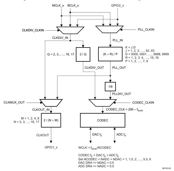
Figure 15. Audio Clock Generation Processing
