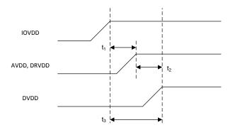
Figure 41. TLV320AIC34 Power Supply Sequencing
