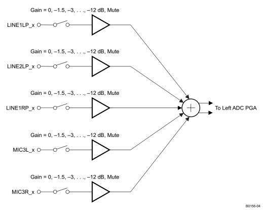
Figure 21. Left-Channel Single-Ended Analog Input Mixing Configuration
