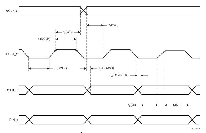
Figure 3. I<sup>2</sup>S, LJF, RJF Timing in Slave Mode
