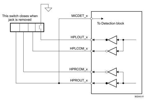
Figure 28. Configuration of Device for Jack Detection Using a Fully Differential Stereo Headphone Output Connection
