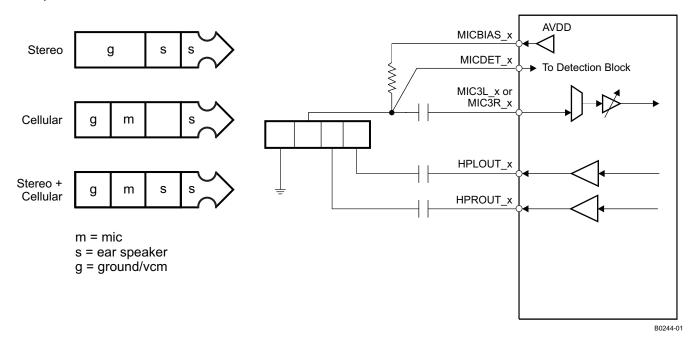
Figure 27. Configuration of Device for Jack Detection Using an AC-Coupled Stereo Headphone Output Connection
