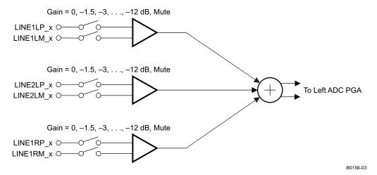
Figure 20. Left-Channel Fully Differential Analog Mixing Capability
