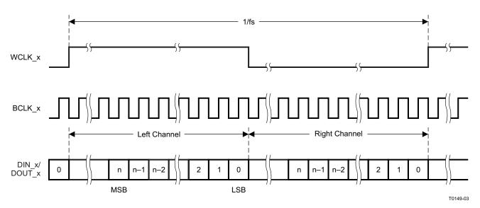
Figure 32. Right-Justified Serial Bus Mode Operation
