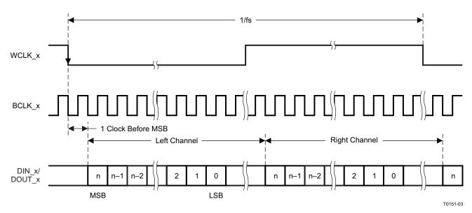
Figure 34. I<sup>2</sup>S Serial Data Bus Mode Operation
