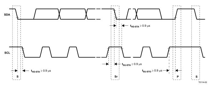
Figure 29. I<sup>2</sup>C Fast-Mode Timing Requirements
