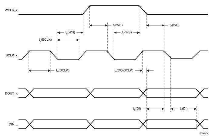
Figure 4. DSP Timing in Slave Mode
