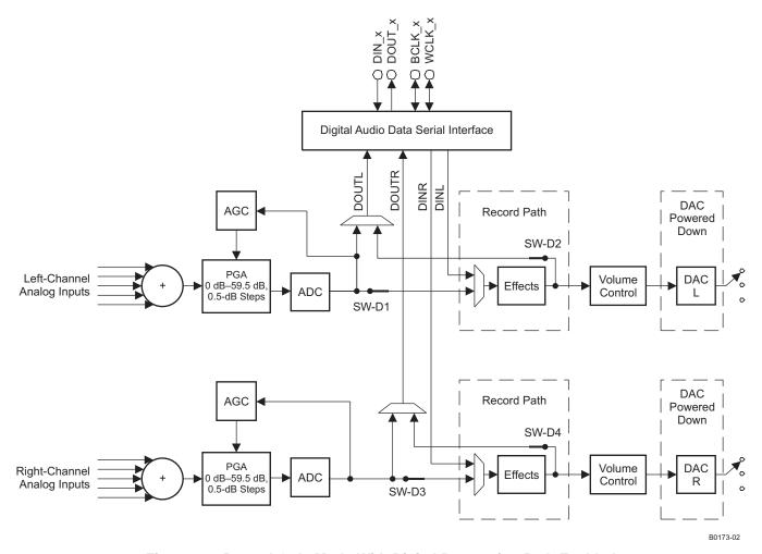
Figure 16. Record-Only Mode With Digital Processing Path Enabled
