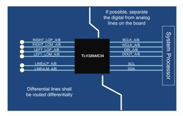
Figure 43. Analog Digital Lines
