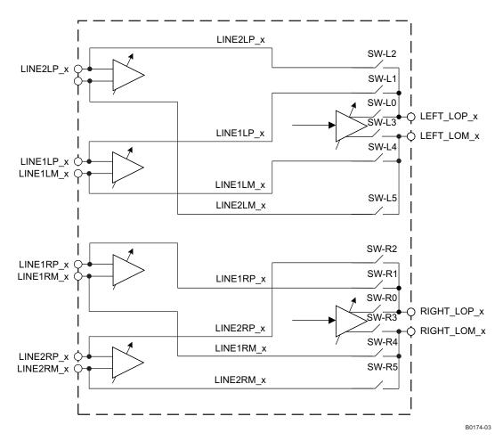
Figure 22. Passive Analog Bypass Mode Configuration
