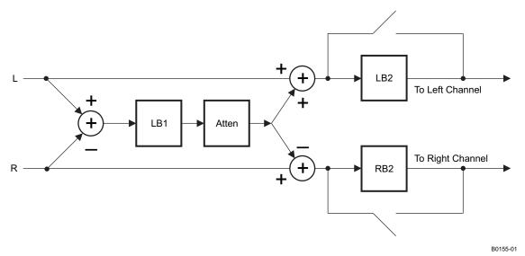
Figure 19. Architecture of the Digital Audio Processing When 3-D Effects are Enabled
