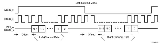
Figure 14. DSP Mode and Left-Justified Mode Showing the Effect of a Programmed Data Word Offset
