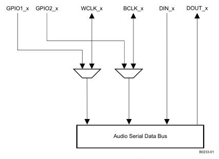
Figure 13. Internal Multiplex Capability on Each I<sup>2</sup>S Bus, Enabling Communication With Multiple External Devices
