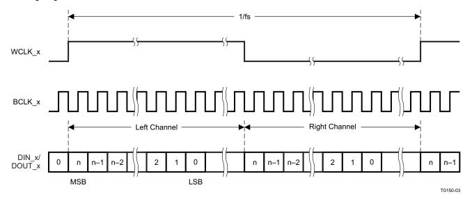
Figure 33. Left-Justified Serial Data Bus Mode Operation
