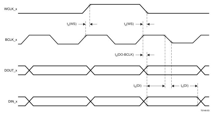
Figure 2. DSP Timing in Master Mode
