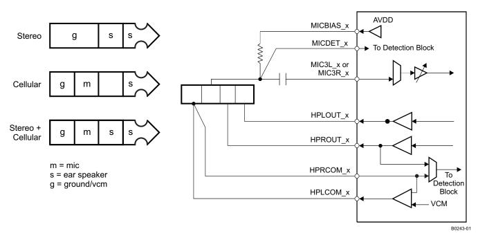
Figure 26. Configuration of Device for Jack Detection Using a Pseudo-Differential (Capless) Headphone Output Connection
