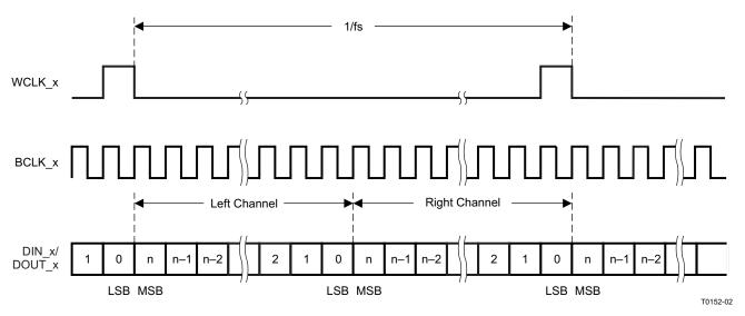
Figure 35. DSP Serial Bus Mode Operation
