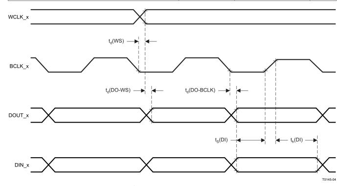
Figure 1. I<sup>2</sup>S, LJF, RJF Timing in Master Mode
