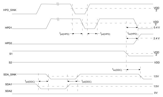
Figure 7. Port Switch Timing Definitions
