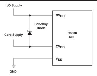
Figure 11. Schottky Diode Diagram
