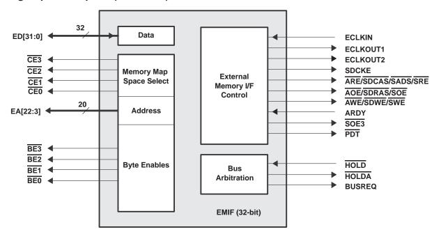
Figure 4. Peripheral Signals
