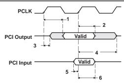
Figure 49. PCI Intput/Output Timing
