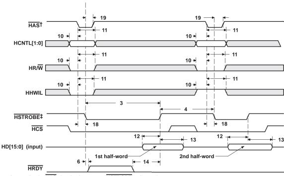
Figure 42. HPI16 Write Timing (HAS Used)
