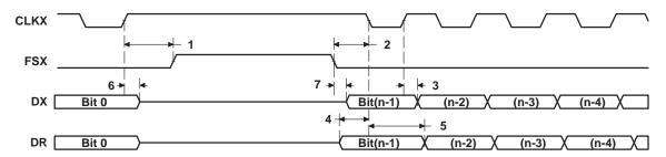
Figure 56. McBSP Timing as SPI Master or Slave: CLKSTP = 11b, CLKXP = 1
