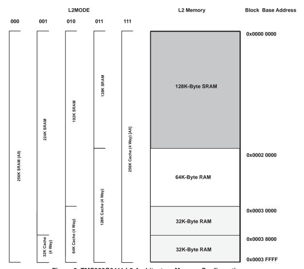
Figure 2. TMS320C6411 L2 Architecture Memory Configuration
