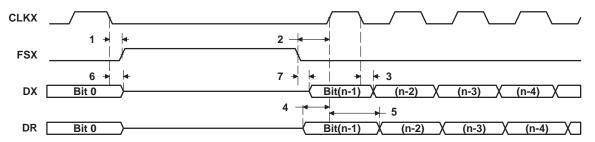
Figure 54. McBSP Timing as SPI Master or Slave: CLKSTP = 11b, CLKXP = 0
