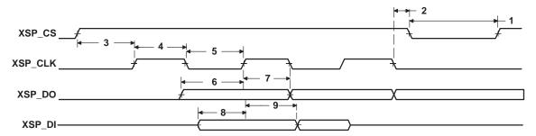
Figure 50. PCI Serial EEPROM Interface Timing
