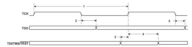
Figure 59. JTAG Test-Port Timing
