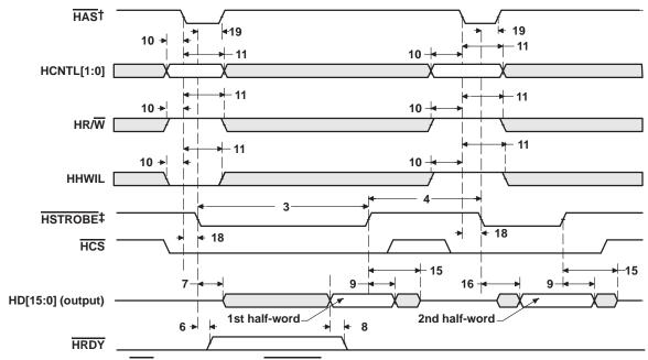
Figure 40. HPI16 Read Timing (HAS Used)
