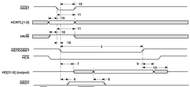
Figure 44. HPI32 Read Timing (HAS Used)
