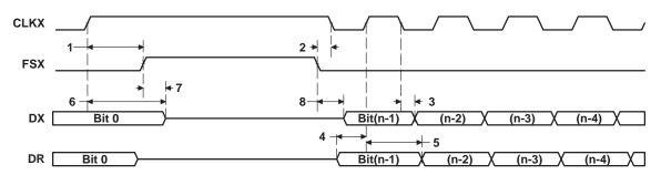
Figure 55. McBSP Timing as SPI Master or Slave: CLKSTP = 10b, CLKXP = 1
