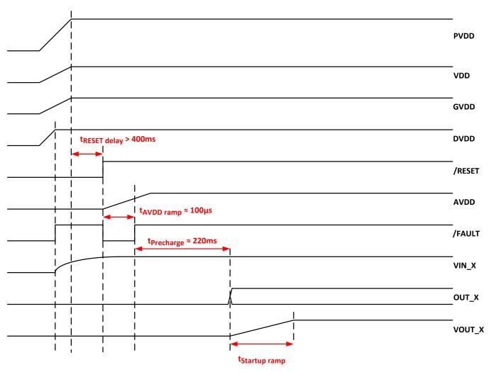
Figure 25. Startup Timing
