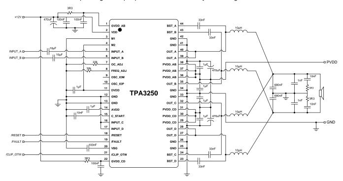
Figure 24. Typical Differential (2N) PBTL Application
