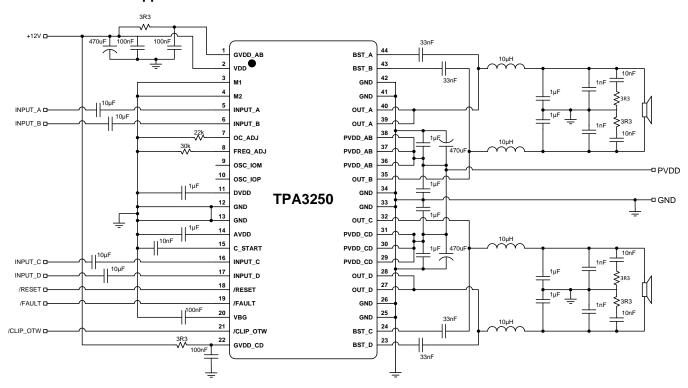
Figure 22. Typical Differential Input BTL Application
