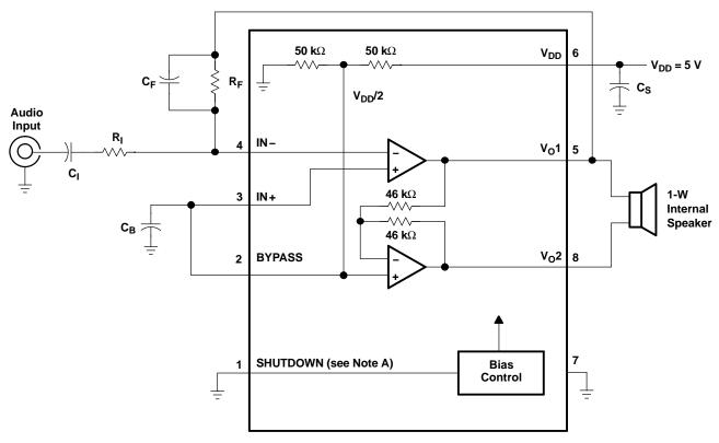
NOTE A: SHUTDOWN must be held low for normal operation and asserted high for shutdown mode.
