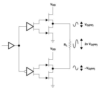
Figure 34. Bridge-Tied Load Configuration
