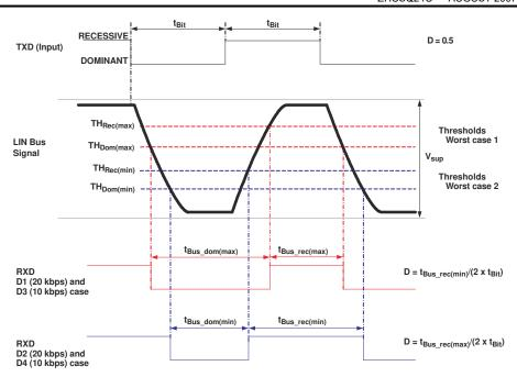
图 8-1. Definition of Bus Timing Parameters
