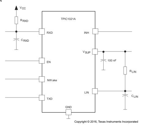
图 9-1. Test Circuit for AC Characteristics
