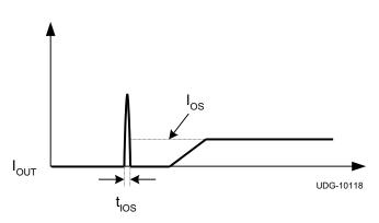
图 31. Response Time to Short-Circuit Waveform
