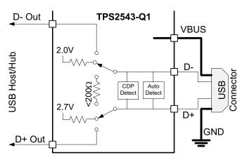
Figure 30. Divider2 Charging Scheme
