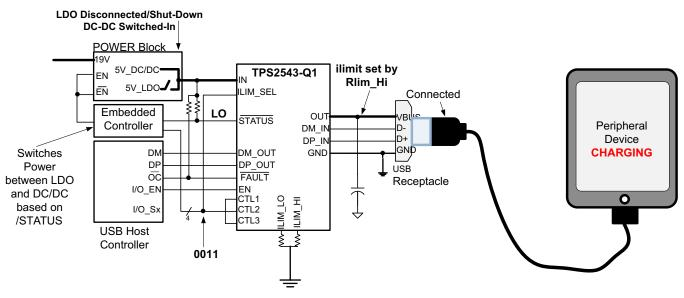
Figure 35. Case 1: System in S4/S5, Device Charging
