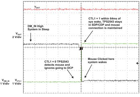
Figure 33. Mouse Wake from Sleep Scope Plot
