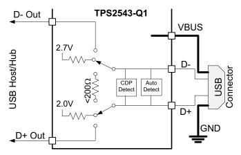
Figure 29. DCP Divider1 Charging Scheme
