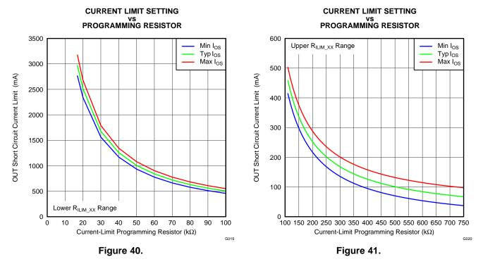
The traces routing the  $R_{ILIM_XX}$  resistors should be a sufficiently low resistance as to not affect the current-limit accuracy. The ground connection for the  $R_{ILIM_XX}$  resistors is also very important. The resistors need to reference back to the TPS2543-Q1 GND pin. Follow normal board layout practices to ensure that current flow from other parts of the board does not impact the ground potential between the resistors and the TPS2543-Q1 GND pin.
