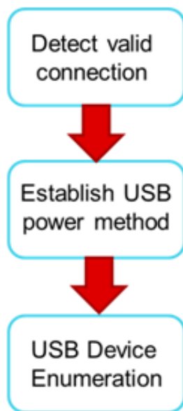
图 11. Flow of DFP to UFP Configuration
