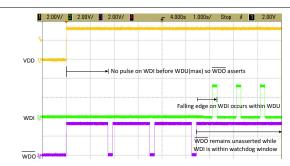
图 8-5. WDO Fault Caused by missing WDI Pulses Followed by Correct Timing WDI Pulses
