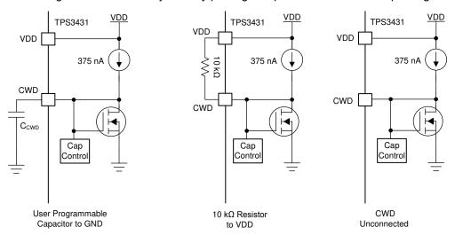
图 8-1. CWD Charging Circuit
