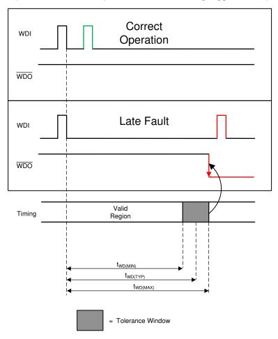
图 7-1. Watchdog Timing Diagram
