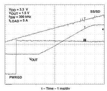
Figure 21. Start-Up Operation Without Transient Comparators
