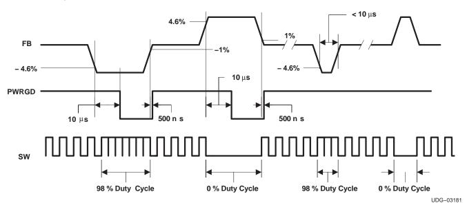
Figure 7. Duty Cycle Waveforms
