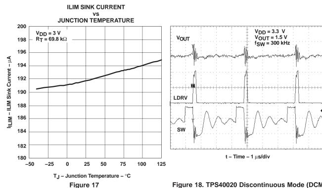
Figure 18. TPS40020 Discontinuous Mode (DCM)
