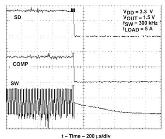
Figure 24. COMP Shutdown Operation
