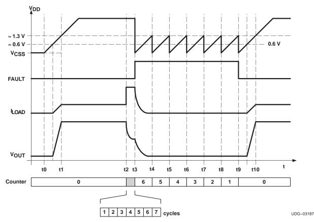
Figure 4. Overcurrent/Fault Waveforms
