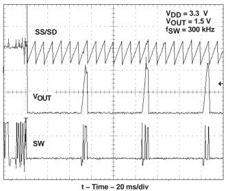
Figure 20. Output Current Fault Operation
