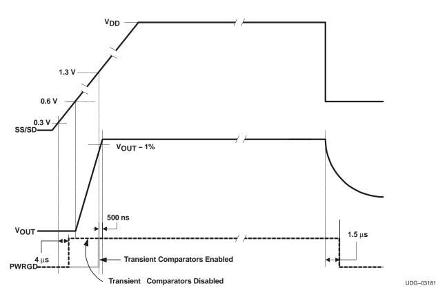
**Figure 8. Transient Comparator Waveforms**
