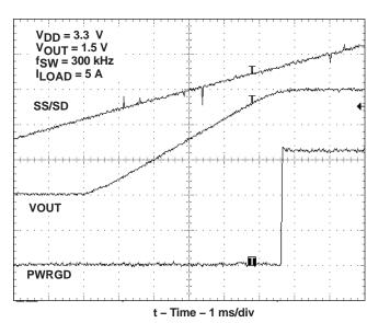
Figure 23. Start-Up Operation With Transient Comparators
