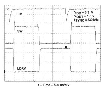
Figure 25. PWRGD Shutdown Operation
