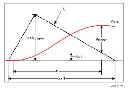
Figure 6. DCM V<sub>OUT</sub> Ripple Calculation
