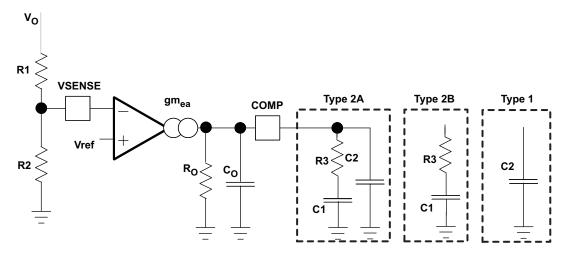
Figure 33. Types of Frequency Compensation
