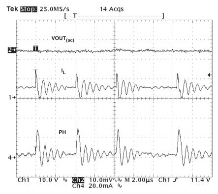
Figure 25. Pulse Skip Mode Operation
