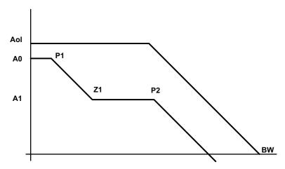
Figure 34. Frequency Response of the Type 2A and Type 2B Frequency Compensation
