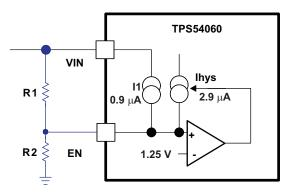
Figure 35. Adjustable Undervoltage Lockout (UVLO)
