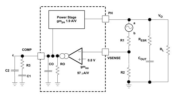
Figure 31. Small Signal Model for Loop Response
