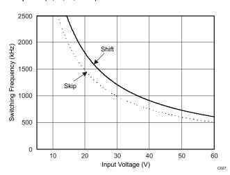
Figure 45. Maximum Switching Frequency vs Input Voltage
