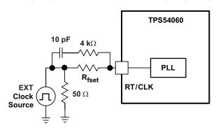
Figure 46. Synchronizing to a System Clock
