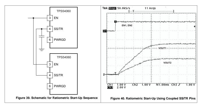
Figure 39 shows a method for ratio-metric start up sequence by connecting the SS/TR pins together. The regulator outputs will ramp up and reach regulation at the same time. When calculating the slow start time the pull up current source must be doubled in Equation 1. Figure 40 shows the results of Figure 39.
