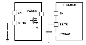
Figure 37. Schematic for Sequential Start-Up Sequence
