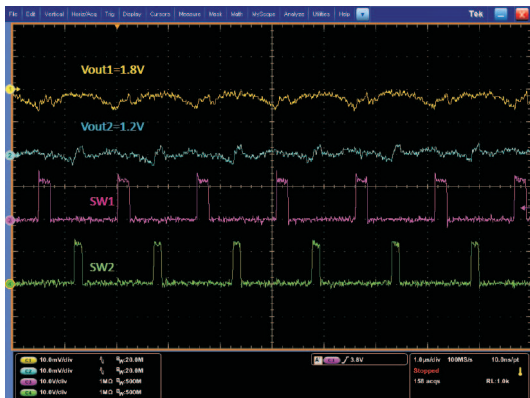
Figure 7. Buck 1 and Buck 2 in Steady State I_{O1} = 0\text{ A} , I_{O2} = 0\text{ A}
