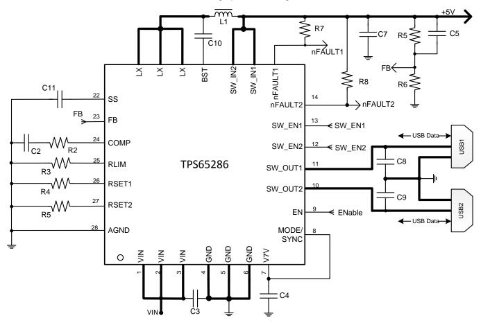
Figure 31. Typical Application Schematic
