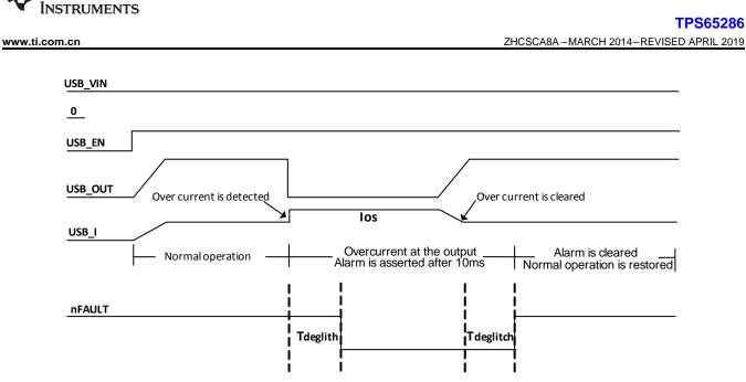
Figure 22. USB Switch Over Current Operation
