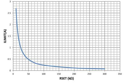
Figure 23. Current-Limit Threshold I<sub>OS</sub> vs RLIM
