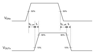
Figure 1. Power Switches Test Circuit and Voltage Waveforms
