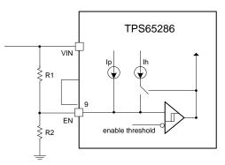
Figure 26. Adjustable VIN Under Voltage Lock Out
