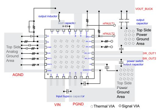
Figure 62. 4-Layers PCB Layout Recommendation Diagram
