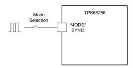
Figure 25. Clock Synchronization Mode
