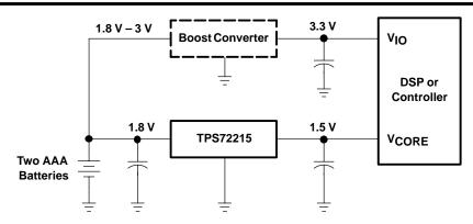
Figure 17. Dual Supply Application Circuit
