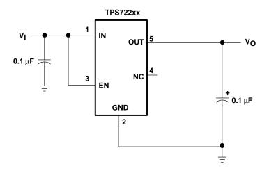
Figure 16. Typical Application Circuit
