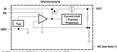
(1) This pin must be left floating and not connected to  $\ensuremath{\mathsf{GND}}$
