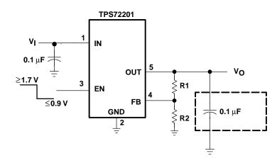
Figure 18. TPS72201 Adjustable LDO Regulator Programming
