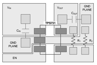
Figure 35. Example Layout (DBV Package)
