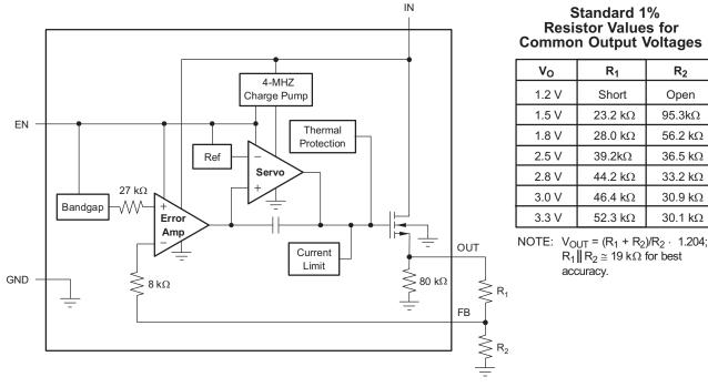
Figure 30. Adjustable-Voltage Version
