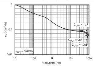
Figure 15. Noise Spectral Density  $c_{NR} = 0 \mu F$
