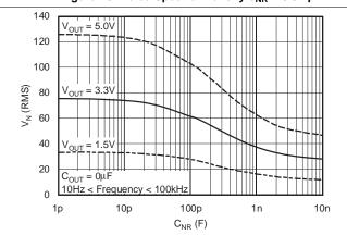
Figure 18. RMS Noise Voltage vs C<sub>NR</sub>
