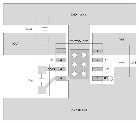
Figure 37. Fixed Output Voltage Option Layout (DRB Package)
