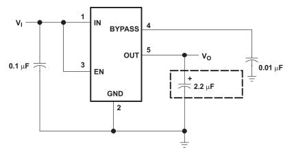
Figure 24. Typical Application Circuit
