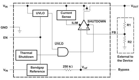
Figure 22. Functional Block Diagram – Adjustable Version
