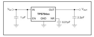
Figure 22. Typical Application Circuit
