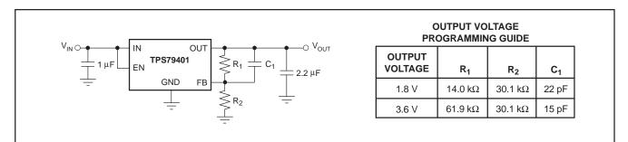
Figure 23. TPS79401 Adjustable LDO Regulator Programming
