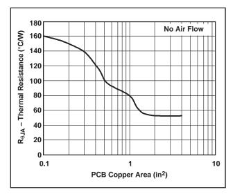
Figure 25. SOT223 Thermal Resistance vs PCB Copper Area
