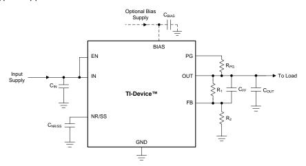
图 47. Typical Application for a 5.0-V Rail
