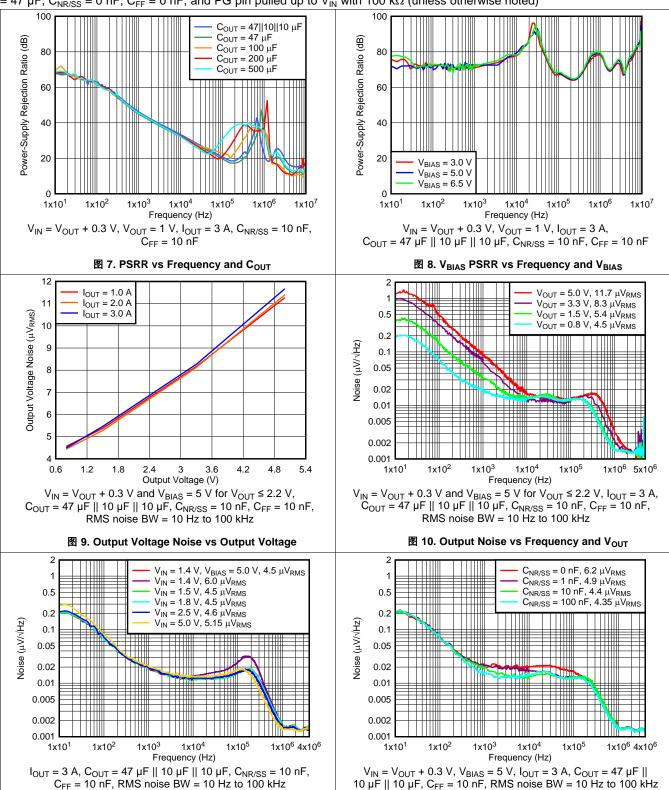
图 11. Output Noise vs Frequency and VIN
