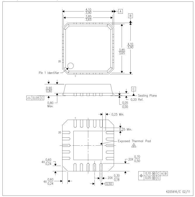
NOTES: A. All linear dimensions are in millimeters. Dimensioning and tolerancing per ASME Y14.5—1994.
