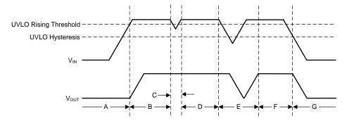
图 44. Typical UVLO Operation
