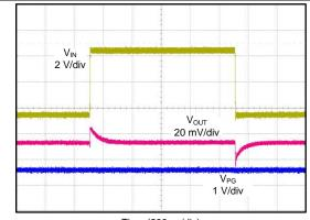
$\begin{aligned} &\text{Time (200 }\mu\text{s/div)}\\ V_{IN} = 1.4 \text{ V to } 6.5 \text{ V to } 1.4 \text{ V at 2 V/}\mu\text{s, V}_{OUT} = 0.8 \text{ V,}\\ I_{OUT} = 1 \text{ A, C}_{NR/SS} = C_{FF} = 10 \text{ nF, V}_{PG} = V_{OUT} \end{aligned}$
