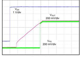
$\begin{aligned} & \text{Time (2 ms/div)} \\ & V_{\text{IN}} = 1.4 \text{ V}, \text{ } V_{\text{PG}} = V_{\text{OUT}} \end{aligned}$
