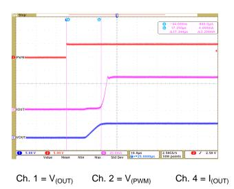
图 20. Output Current With PWM Input
