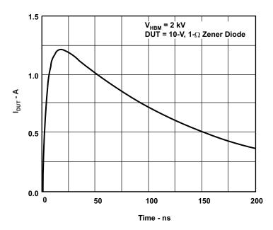
**Figure 6. Typical HBM Current Waveform**
