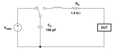
Figure 5. HBM ESD Test Circuit
