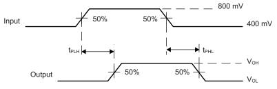
Figure 8. Propagation Delay
